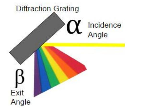
Rearranging to solve for exit angle, we can determine which camera pixel corresponds to a given wavelength. Intensity of each pixel can be determined by averaging neighboring RGB pixels according to the equation: I = 0.2989\*R + 0.5870\*G + 0.1140\*B
