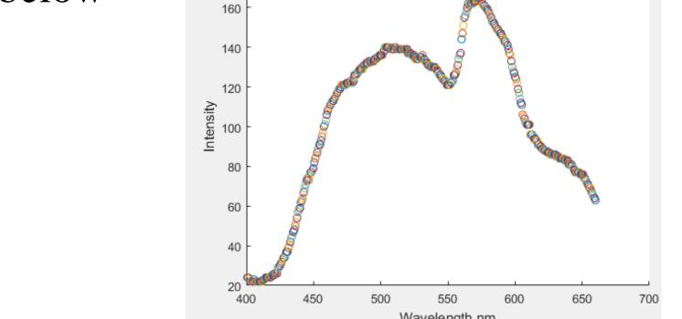
• App performs analysis of baseline vs new intensity spectra to determine substance present on PDMS
