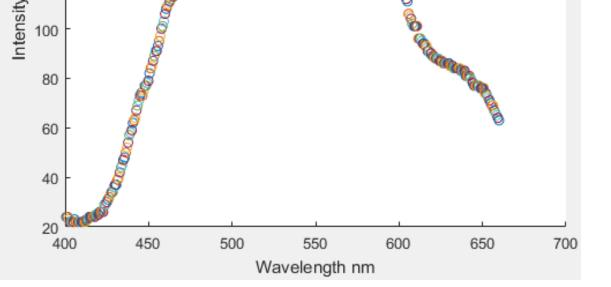
After determining the base state and new intensity spectra of the expanded PDMS, we can determine how much the wavelength changes for each percentage of amount of gas around the PDMS. Doing this several times and using regression we can find how big of intensity increases correspond to gas concentrations in the air.
