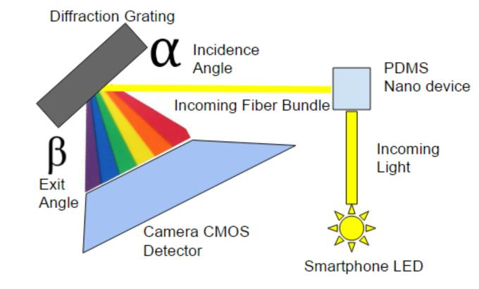
• Smartphone app graphs intensity vs wavelength of the light on the camera as shown below
